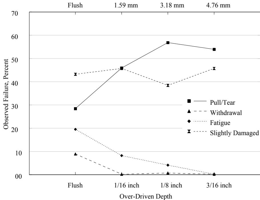
Fig. 1 Nail Failure Trend
